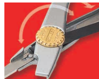
SWIVEL ACTION FOR QUICK BLADE CHANGE.
